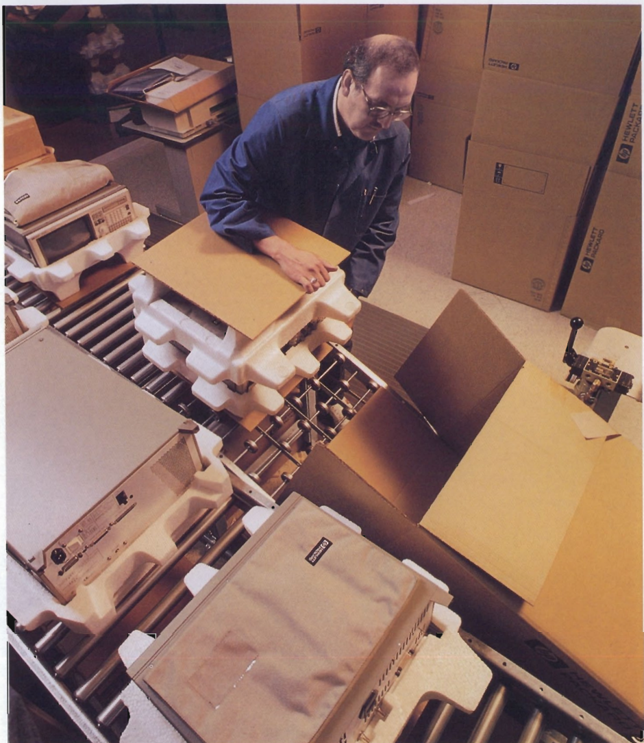
Colorado Springs Division redesigned the packaging process so that operators, such as Chris Montoya, can tilt products and slip them into shipping cartons instead of lifting them.
